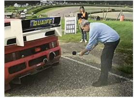
all must within 150mm of the outside of the vehicle but not protrude by more than 4cms. Where a vehicle has two separate exhausts, measurement must be taken of each, with the higher reading taken as the record [not an average]. No temporary silencing parts or material may be added. E.S can refuse test, and car can be disqualified. [J.5.17]
